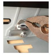
3. With the tab removed as shown in the picture below you can now remove the old lock and insert the new one. Push the tab back into place making sure that the tab seats up against the lock in the grooves on the sides of the lock housing.
